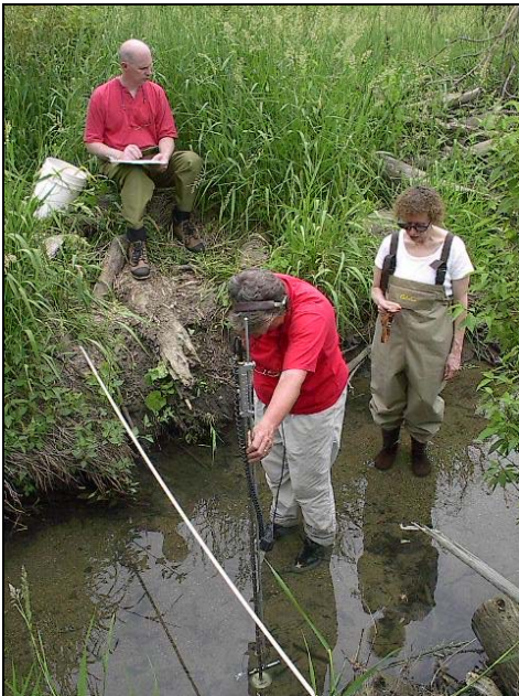
A volunteer team measures and records data for flow measurement on a small stream.
