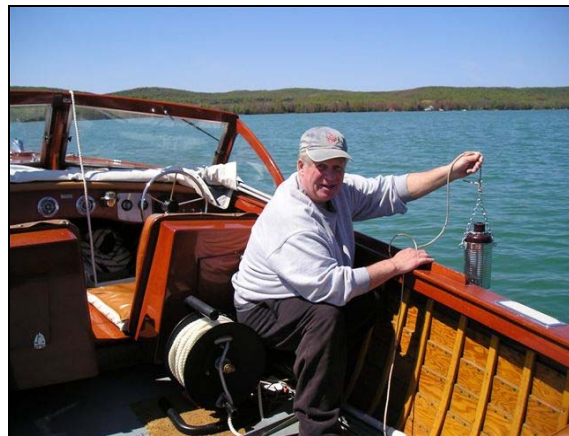
CLMP volunteer Bruce Lichliter, from Big Glen Lake, prepares to take a water sample that will be filtered and sent to the DNRE water quality lab for chlorophyll a analysis.
