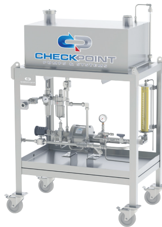
NACE compliant portable 6212 batch treatment injection package with 2507 tubing and fittings, custom fabricated top mounted 35 gallon SS316 chemical tote tank with level gauge and flame arrestor. Final destination: GOM floating drill rig
